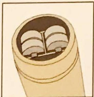
Put the tester in a new pH 7.01 calibration buffer solution and try to calibrate. Then put the tester in a new pH 4.01 calibration buffer solution and try to calibrate. If the calibration cannot be performed the pH electrode has **dried out (A)** or is **dirty (B)** (not being cleaned after use) or maybe **the calibration**
